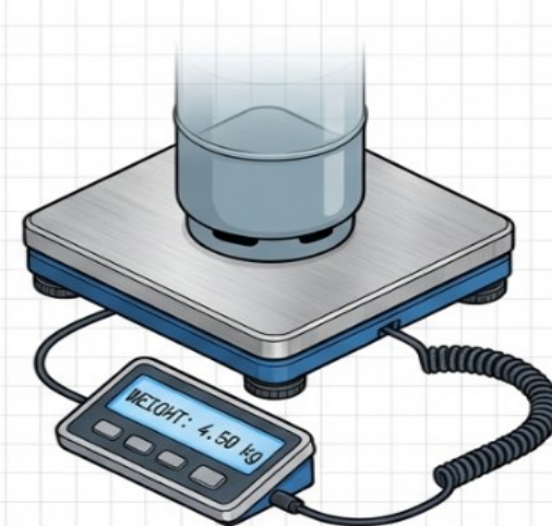
Charging Scale: Mandatory for F-Gas compliance (Weigh-in Charge).
