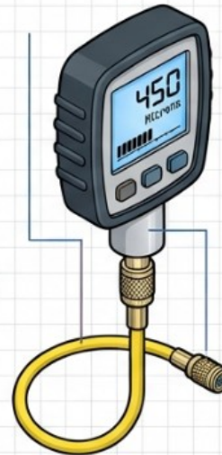
Micron Gauge: Verify deep vacuum (<500 microns) for moisture removal.
